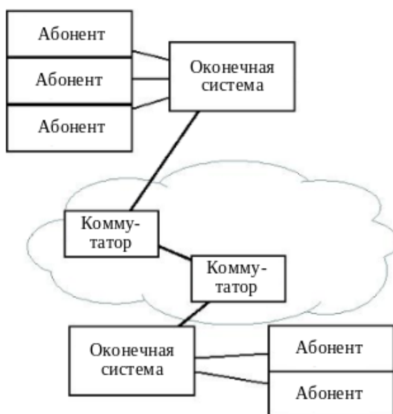
Рис. 2: Типовая структура сети AFDX Figure 2: Typical structure of an AFDX network
