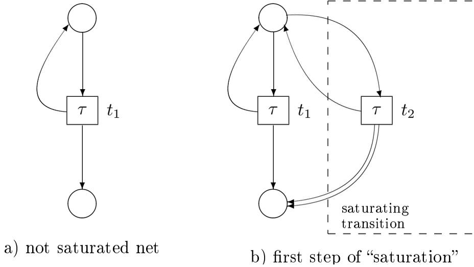
Fig. 5. Not saturable net
