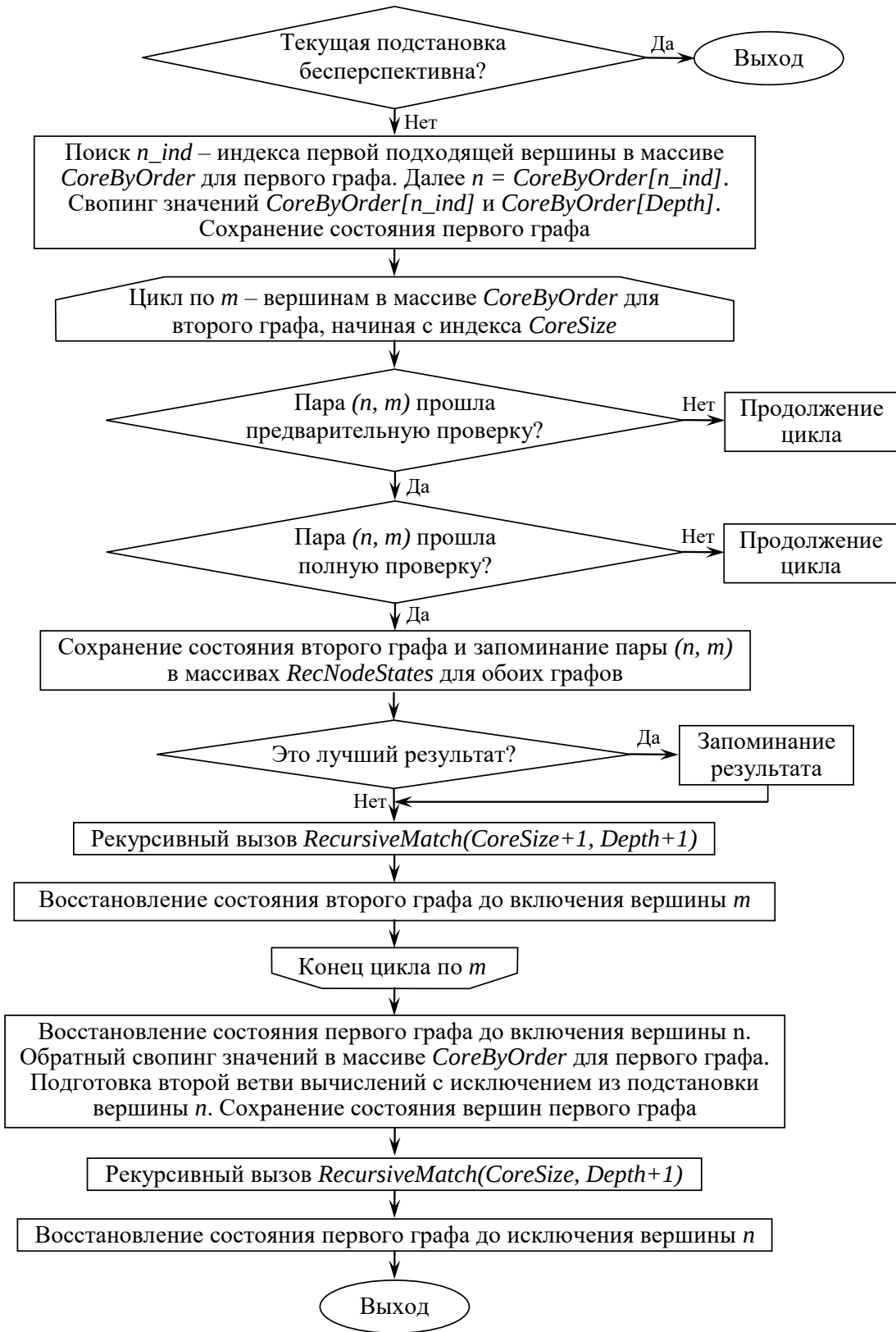
Fig. 1. Block diagram of the serial method RecursiveMatch(CoreSize, Depth)
