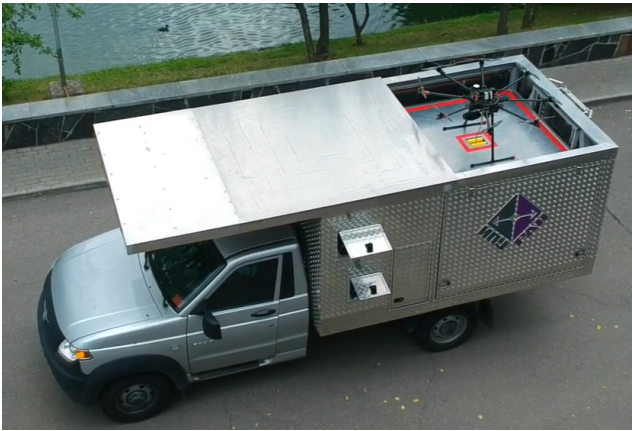
Fig. 1. Tethered high-altitude telecommunication platform "Albatros"
